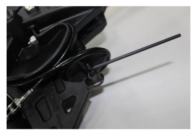
If you look closely at the idler cable pulley you will notice that it is also held in place on its shaft with the same size set screw. Although not as critical as the sprocket shaft set screw, it's probably a good idea to take a quick look at that every now and again as well. Be sure not to over-tighten it. You could use Loctite here also.
