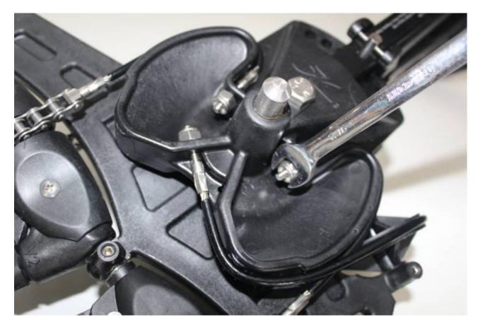
Chain and cable tension is achieved with the 1/4 inch lock nuts at their ends. It might take a turn or two on each nut at both ends of the cables to achieve the desired tension.
