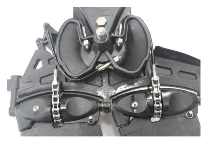
**Rinsing**: The most important thing to remember is that the drive should be rinsed thoroughly with fresh water after use in salt water. In the event that sand has collected in and around the chains and sprockets it's good advice to use a fairly high pressure stream of water to dislodge and remove it.
